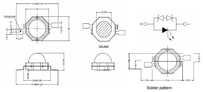
Note: 1. Dimensions are in millimeters
