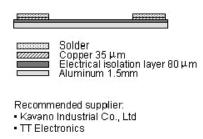
Special thermal designs are also recommended to take in outer heat sink design, such as FR4 PCB on Aluminum with thermal vias or FPC on Aluminum with thermal conductive adhesive, etc. Sufficient thermal management must be conducted, or the die junction temperature will be over the limit under large electronic driving and LED lifetime will decrease critically.
