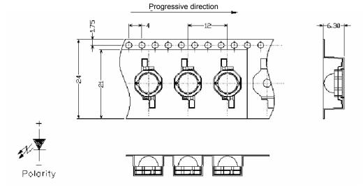
Note: 1. Dimensions are in millimeters
